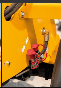
**Evolved and complete hydraulic.**Not only High Flow kit but also additional hydraulic kit for tools and equipments. An example? Hand operated hydraulic demolition hammer!
